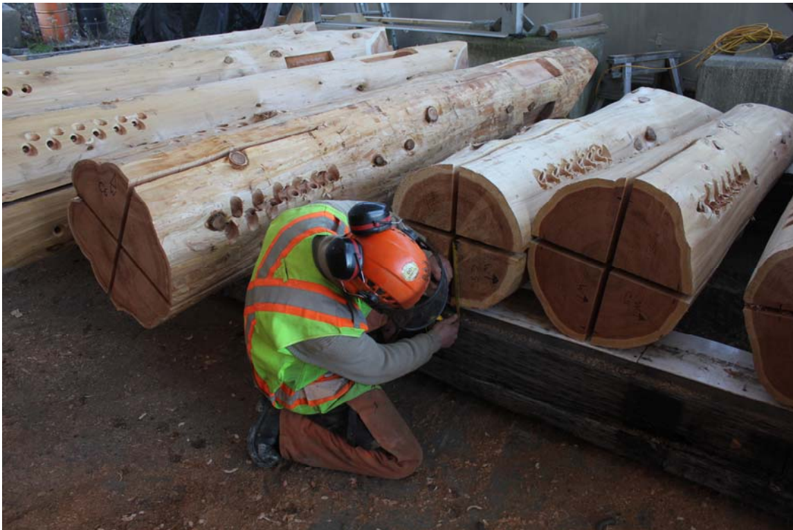
Photo 06: Timber frame: Fabrication: bolt holes
